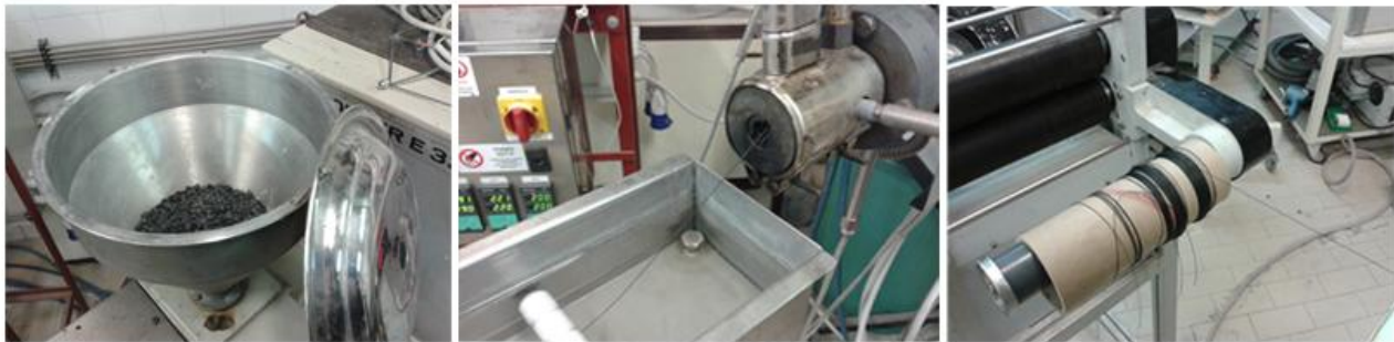
Figure 1: a) Pellets and foaming agent in the hopper; b) single screw extruder die and c) winder collecting foamed strands
