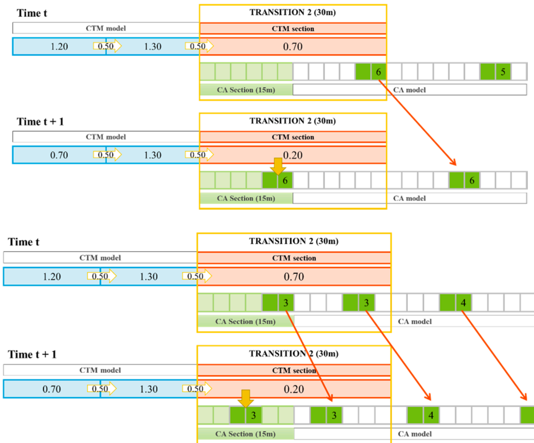
Fig. 17. Transition from CTM to CA with a cumulative transition cell. The numbers in the CA cells are the speeds of the vehicles, while the values on the CTM cells are the number of vehicles.
