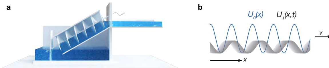
FIG. 1. a Illustration of a classical Archimede's screw (by C. Hohmann, MCQST). b Schematic drawing of two periodic potentials, U_0(x) and U_1(x,t) , that share the same periodicity. One of the two potentials, U_1(x,t) , is moving with a small velocity v with respect to the other in order to realize a quantum pump.
