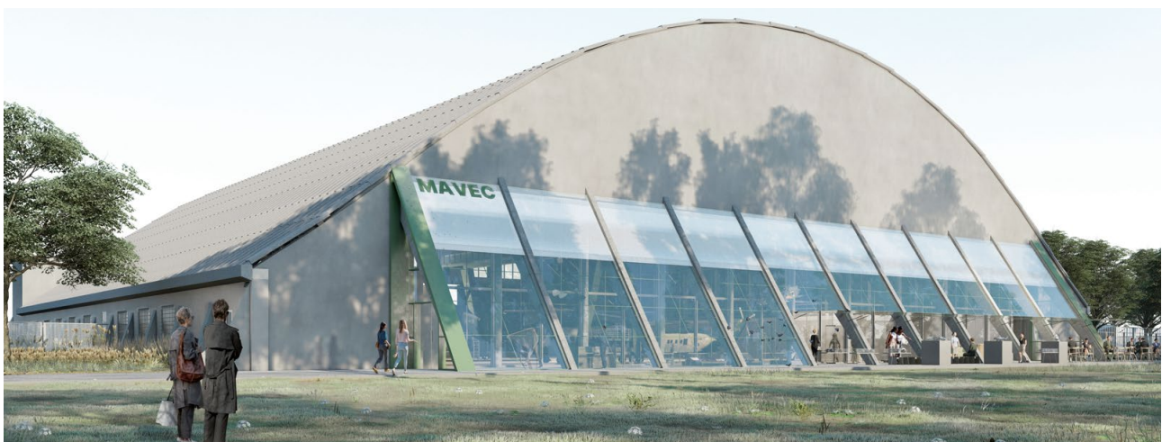
Figure 11 | Intervention on the rear facade of the Hangar in which oblique reinforced concrete elements are preserved and exhibition space created. Source: Design by O. Lopez and G. d'Amato on indication of the authors.
