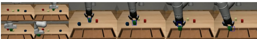
Figure 3.26: Example of unsuccessful Pick-Place rollout. In this case, the robot fails to complete the task due to errors in the bounding box predictions. These inaccuracies cause the robot to move in the wrong direction, leading to an unsuccessful execution of the task.
