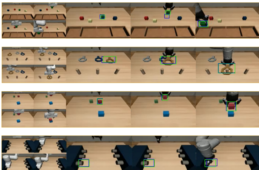
Figure 2.14: Example of predictions generated by the CTOD module in the single-task scenario. The blue-box is the predicted one, while the green is the ground truth.
