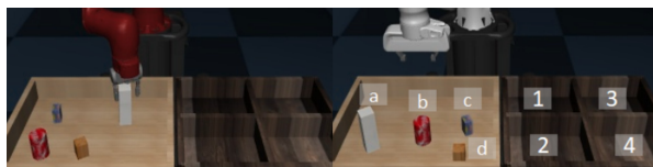
Figure 3.16: Validation setting proposed in [6]. The 16 tasks consist of taking an object (a-b) to a bin (1-4). On the left there is the demonstrator robot, while on the right there is the agent robot.
