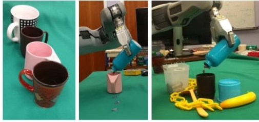
Figure 2.2: Pouring task setting proposed in [107]. (Left) Mugs used for evaluation. Note that only the brown mug was seen during training. Center: Successful pouring into the pink mug. (Right) Pouring into the brown mug in a cluttered environment that was not seen during training.
