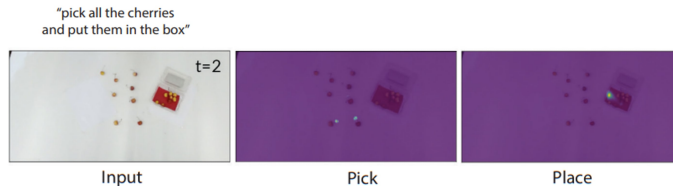
Figure 3.13: Example of affordance map. (Left) The top-view input image. (Center) The affordance map for the pick-operation, since the task is to grab cherries the map highlights the two pickable cherries. (Right) The affordance map for the place operation.
