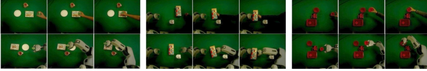
Figure 3.3: Tasks performed in [14]. (Top row) Human demonstration, (Bottom row) robot demonstration. (Left) Placing task, (Middle) pushing task, (Right) pick-and-place task.
