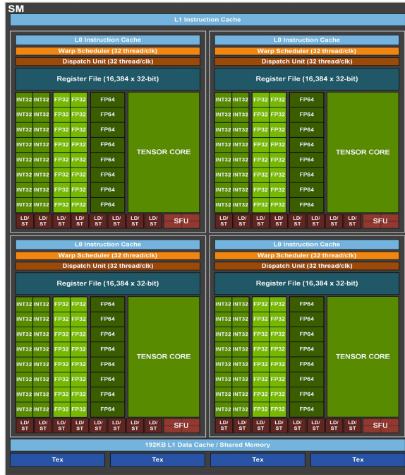
Figure 2.4: The structure of an NVIDIA A100 SM
