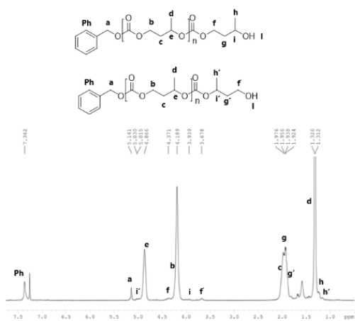
Figure 3.27: ^1\text{H-NMR} spectrum of poly-methyl-trimethylenecarbonate (Solvent: \text{CDCl}_3 , 600 MHz, 25 ^\circ\text{C} ).
