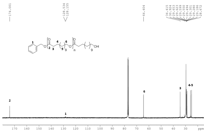
Figure 6.14: ^{13}\text{C} -NMR spectrum of poly(PDL) with benzyloxy and hydroxylic terminal groups (Solvent \text{CDCl}_3 , 100 MHz, 20 °C).
