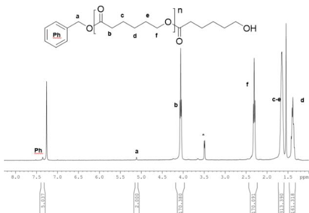
Figure 4.20: ^1\text{H} NMR spectrum of polycaprolactone (solvent: \text{CDCl}_3 , 400 MHz, 25^\circ\text{C} ) * = methanol.
