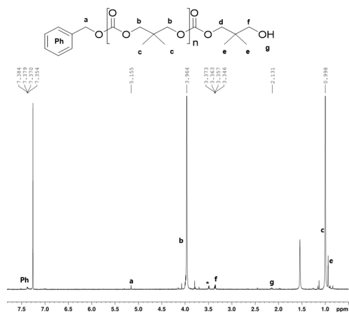
Figure 2.23 ^1\text{H-NMR} spectrum of the poly-2,2'-dimethyl-trimethylenecarbonate (solvent: \text{CDCl}_3 , 300 MHz, 25°C, Entry 19 of Table 2.2 ) *methanol.
