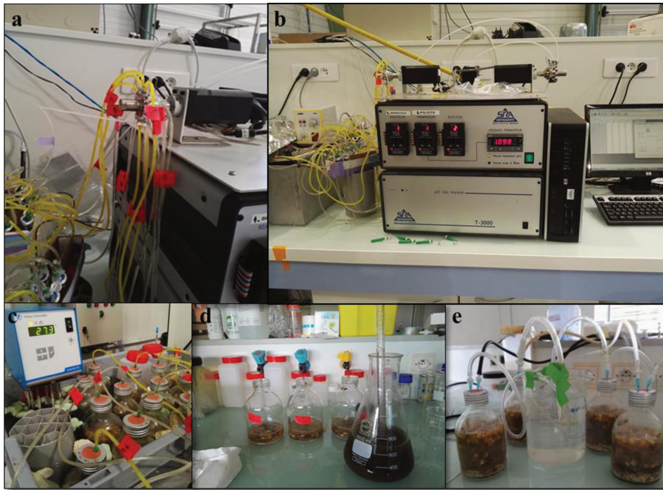
Figure 6-4: Multiplexing the channels (a), conductivity detector of the micro-gas chromatograph (SRA Instrument) (b), water bath equipped with thermostat (c), inoculum (d), purging with nitrogen gas (e)
