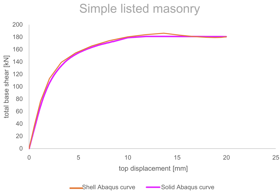
Fig. 25. Comparison between Abaqus “Solid” and “Shell” curves for simple listed masonry in shear.
