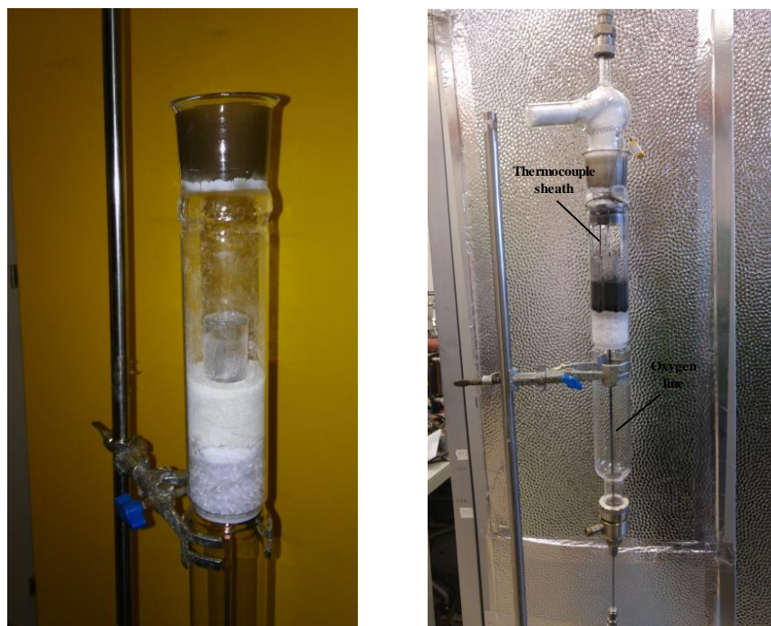
Figure IV. 4 Picture of the quartz reactor loaded with the fresh sample (right) and with the same sample after a stability test (left).
