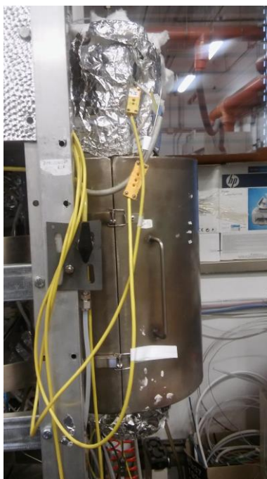
Figure IV. 3 Picture of the electrical oven (right) and scheme of the quartz reactor (left).
