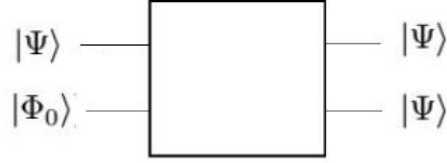
Figure A.1: Cloning machine which starts in the state |\Phi_0\rangle and creates a copy of the state |\Psi\rangle . The box represents the unitary transformation U which acts on both subsystems.
