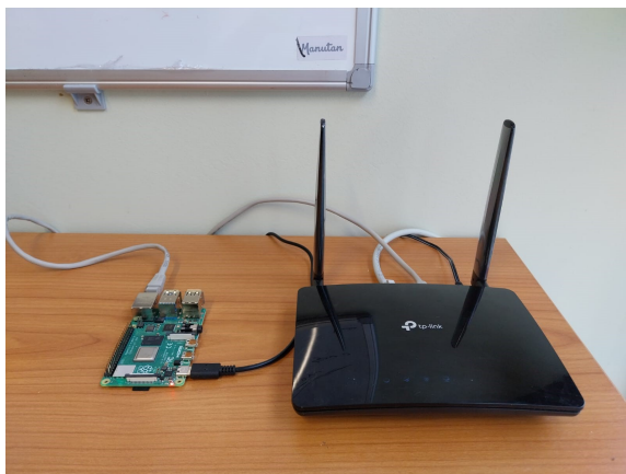
Figure 8.2: Raspberry Pi unit connected to a router, serving as a central hub for smart home automation and energy monitoring tasks.
