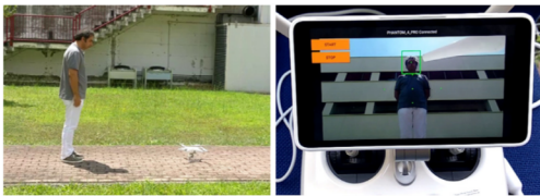
Fig. 4. (Left) The drone is in loop until a face is detected in the scene. (Right) The drone has detected a face and is preparing to take off.
