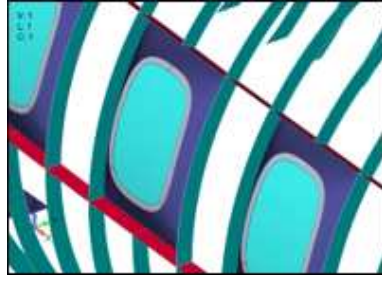
(a) Structural modelling of stringers and frames around a window frame
