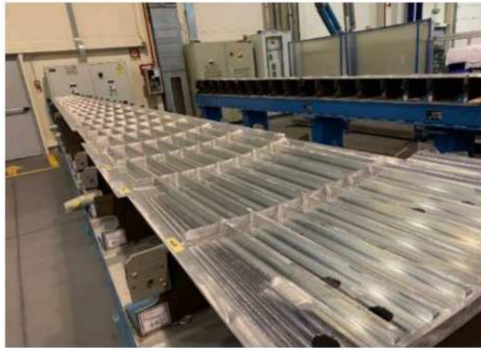
Fig. 3.4 Integrally stiffened machined wing upper panel.
