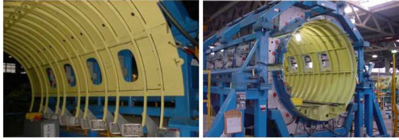
Fig. 3.5 Avanti vacuum jigs for central fuselage assembly.
