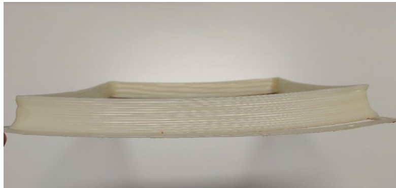
Figure 1-6. Printed part made from pure PA6. Excessive shrinkage prevented successful fabrication of the part
