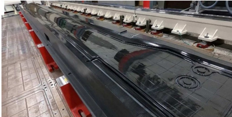
Figure 0-4. 3D printed tool, machined and vacuumed sealed, for fabrication of helicopter's rotor blade [1], [19]
