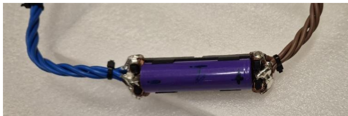
Figure III.14 Real reference 1500 mAh LTO cell
