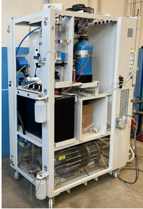
Figure 2.2: Example of a commercial electrolyser unit.
