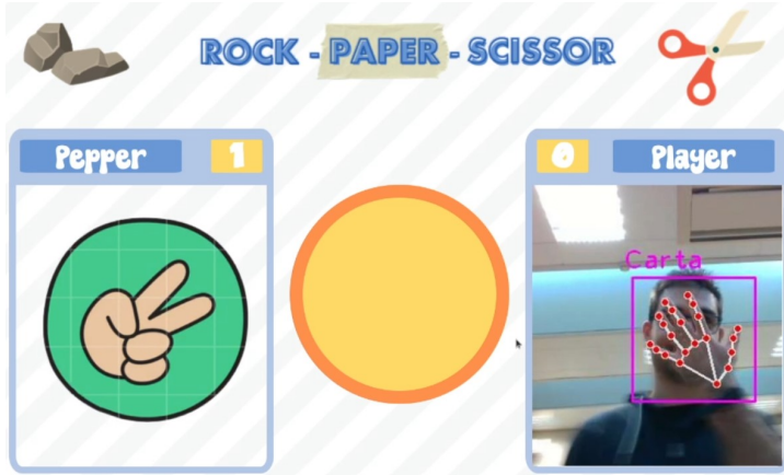
Figure 3.14: Tablet view during the game session. The right side displays the video feed captured by the camera, along with the detected game move chosen by the user (in this specific case it is paper). On the left side, the option selected by the proposed system is shown, which is scissors in this case.
