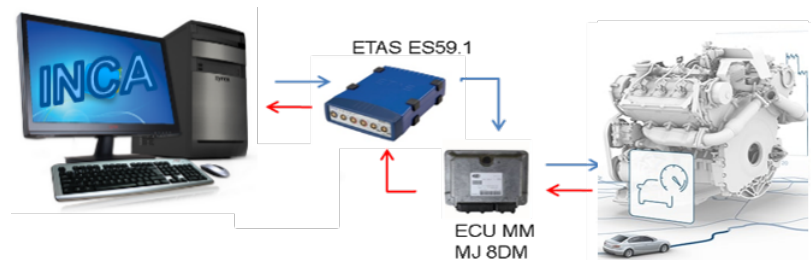
Figure 4-8 Communication scheme between user and engine. Actuation line in blue: input engine variables set by the user; Acquisition line in red: feedback on control strategies from the engine.
