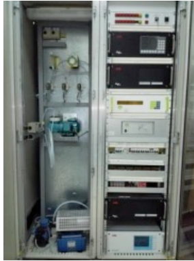
Figure 4-5 Gas analyzer box. On the left side the sampling pump, on the right side the control module (Advance Optima) and the different gas modules.
