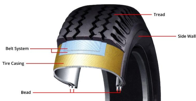
Figura 7 - Parts of a tyre
