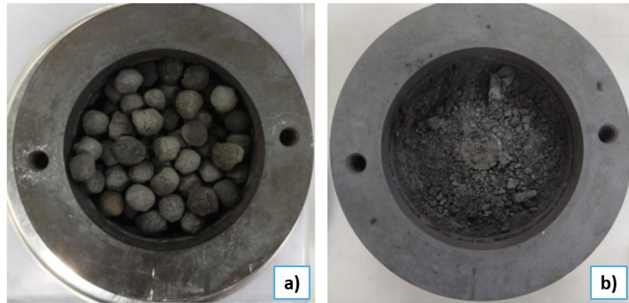
Figure IV.26 Photographic images of the sample containing reduced pellets: (a) before the test; (b) after the test.
