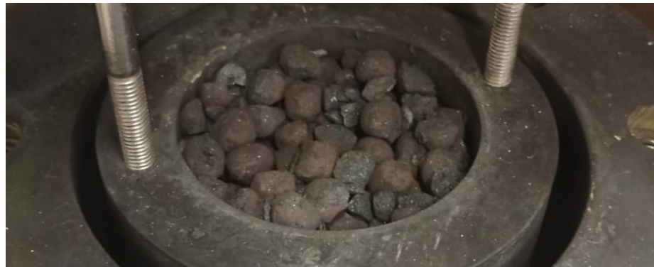
Figure IV.22 Photographic image of the iron oxide sample at the end of the shear test.
