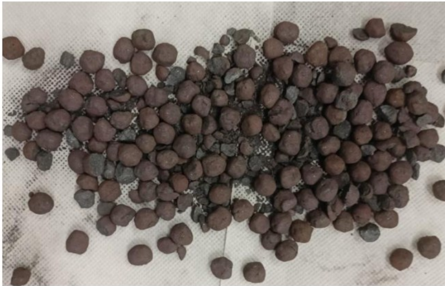
Figure IV.24 Photographic image of the sample downstream of the shear tests, where the effects of fragmentation are evident.
