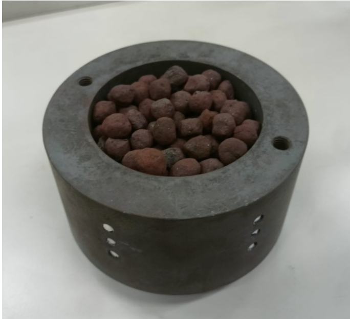
Figure IV.20 Photographic image of the trough filled with 10–13 mm iron oxide pellets after the sample preparation procedure.
