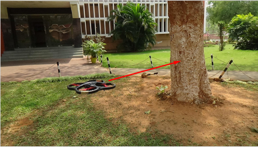
Fig. 1. UAV navigating towards a tree (obstacle). As the UAV moves further, the depth value keeps on decreasing.
