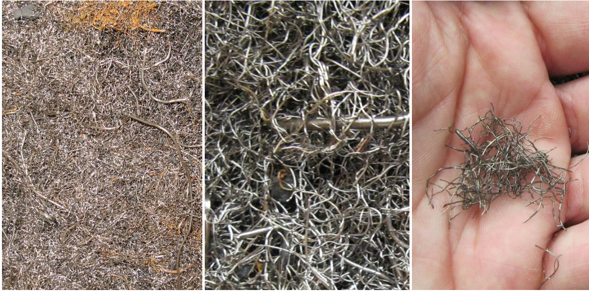
Figure 1: Recycled steel fibers derived from waste tires.
