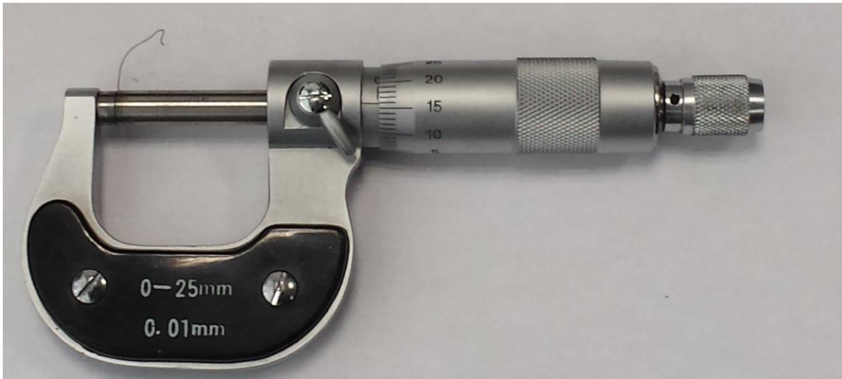
Figure 2: Characterization of fibers: micrometer for the diameter measurements.
