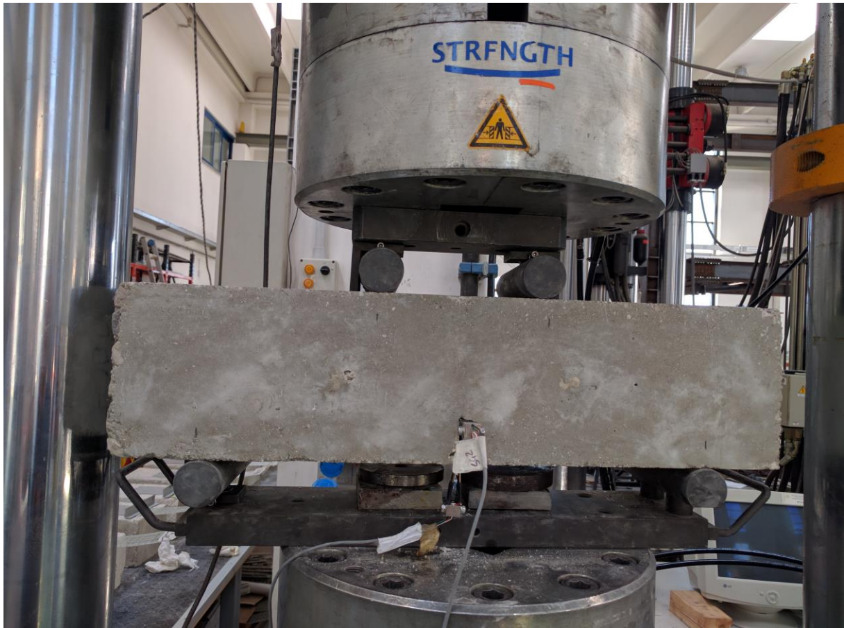
Figure 8: Experimental set-up of the four-point bending test.
