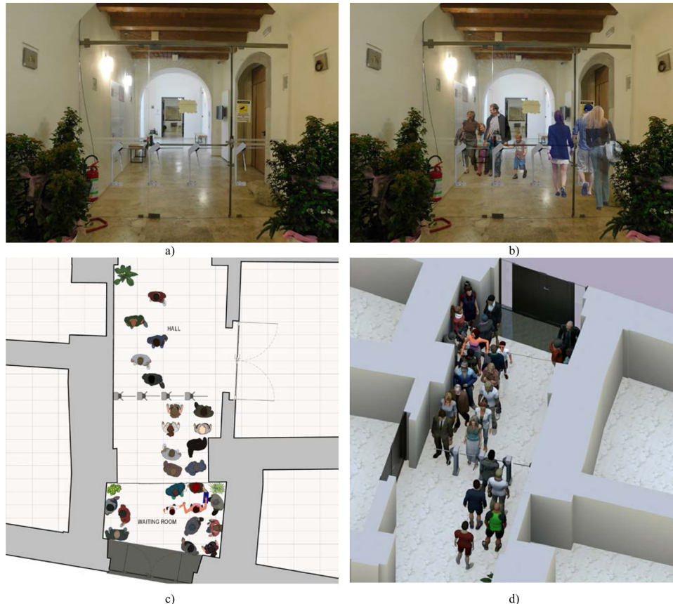
Fig. 10. Proposal of re-organization of the existing hall of the museum with turnstiles (two for entering, and two for exiting), and waiting area: a, b: photorealistic renders; c, d: micro-simulation snapshots.
