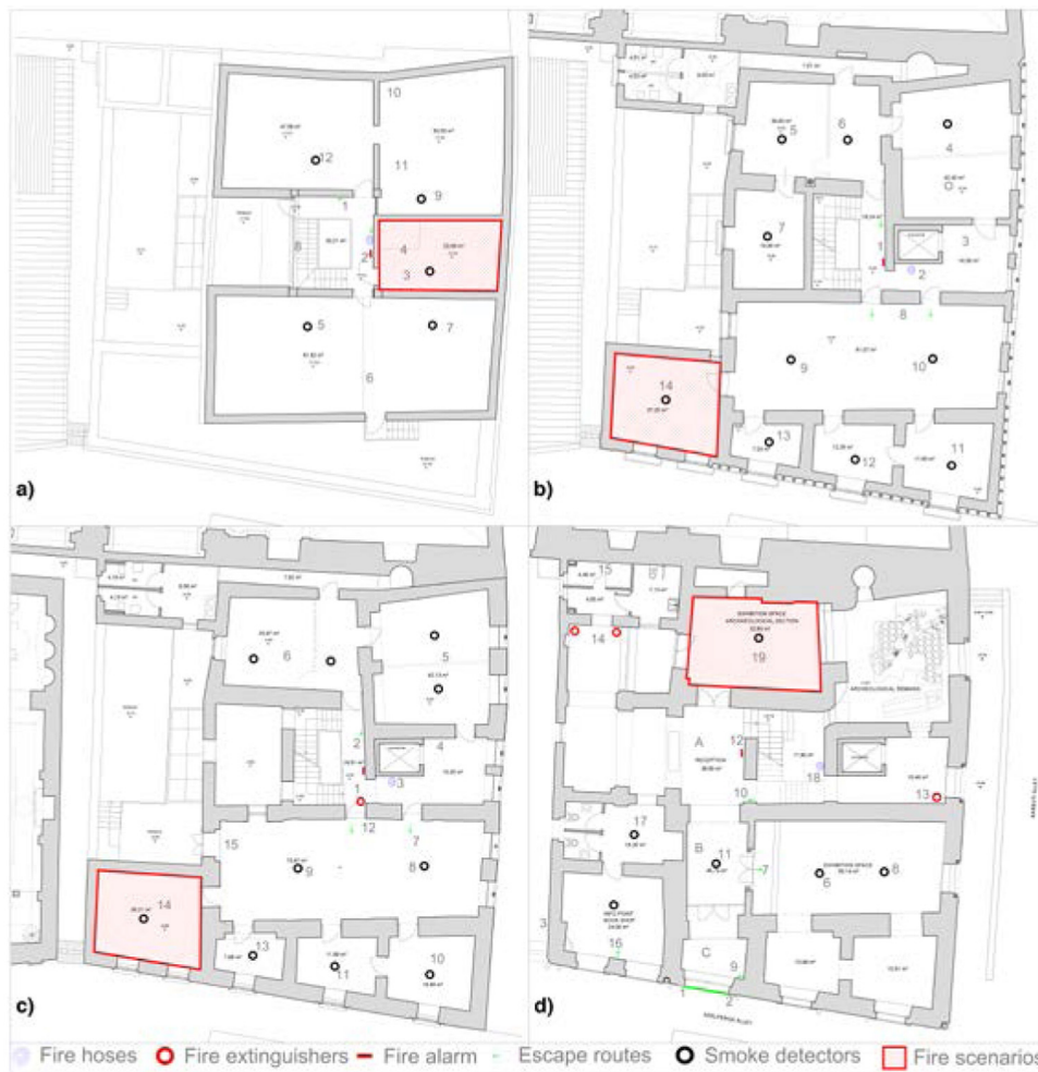
Fig. 4. Building levels and fire scenarios: a: attic (scenario I); b: 2nd floor (scenario II); c: 1st floor (scenario III); d: ground floor (scenario IV).
