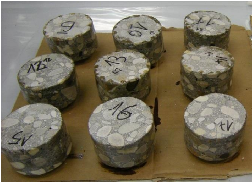
Figure 3: Concrete cylinders used for chloride-ion penetration tests.
