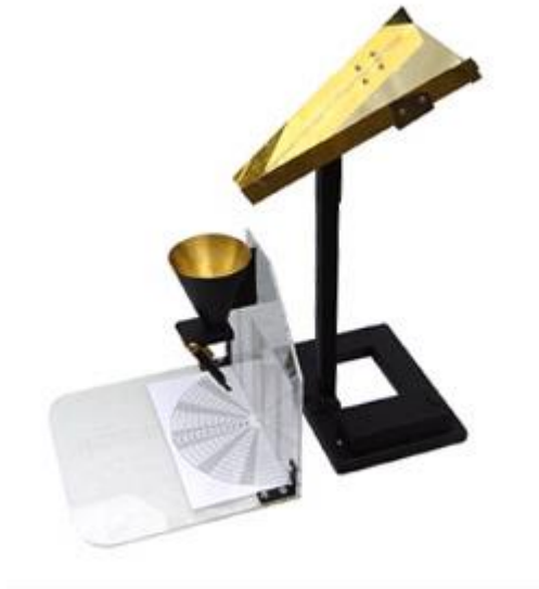
Figure 3. The Geldart apparatus to measure angle of repose [32]
