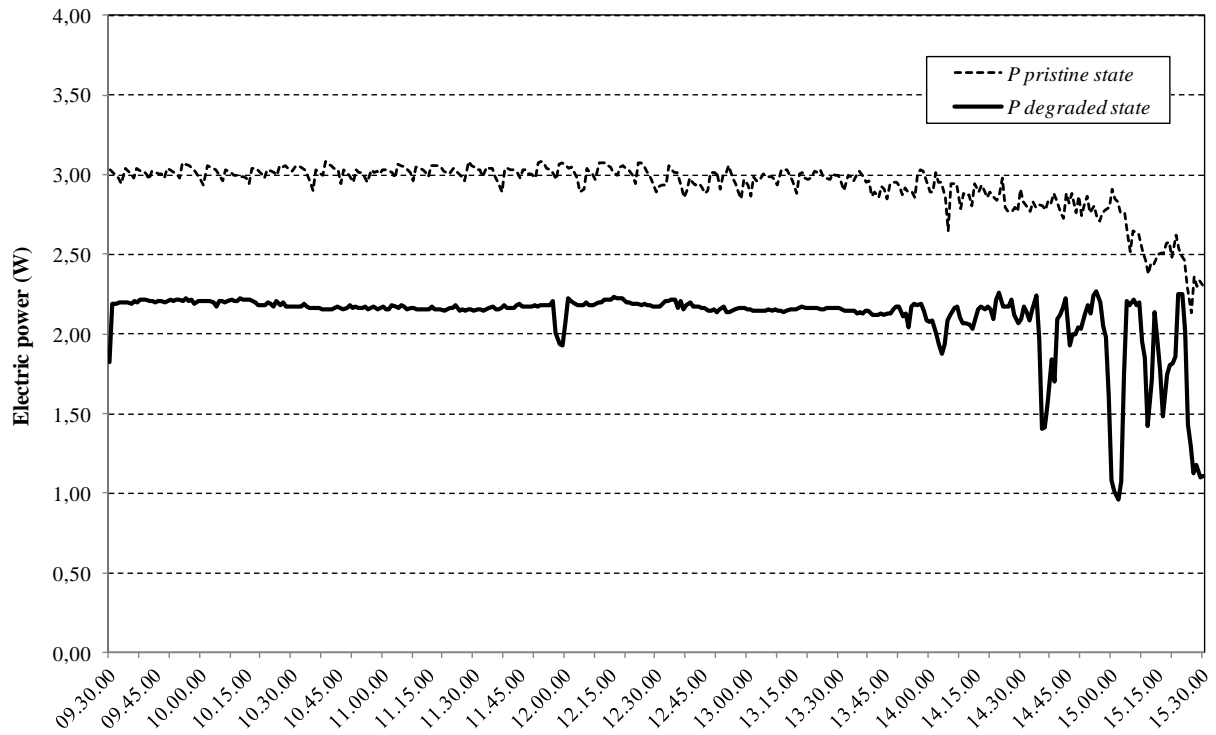
Figure 9 Comparison between the measured electric powers for the TJ solar cell in the pristine and degraded states
