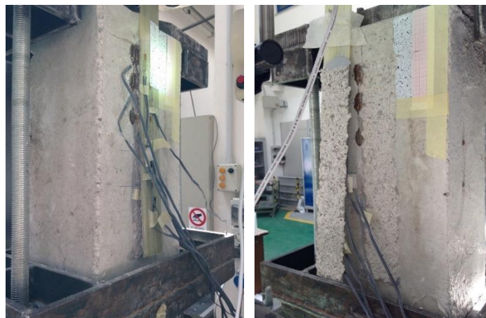
Figure 7. Post mortem fracture surfaces of the specimen #1
