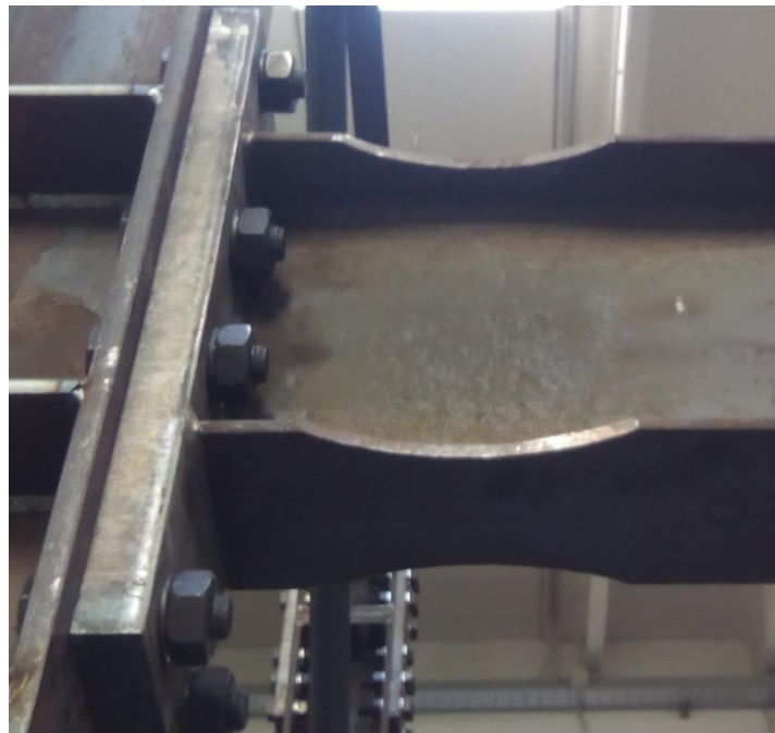
Figure 1: Typical shape of a “Dog-Bone” connection
