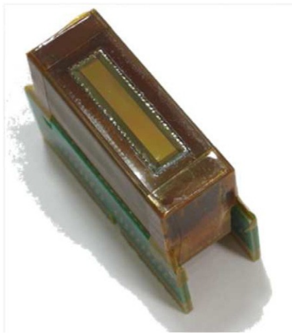
Figure 10. Image of a CMUT array bonded to a rigid-flex PCB and provided with a backing material.
