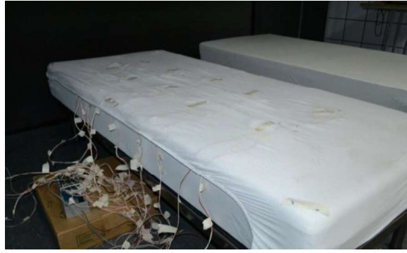
Fig. 2. Location of RTDs on the mattress pad material (on the left, under the thin cover) and their corresponding position on the subject's skin (red points).
