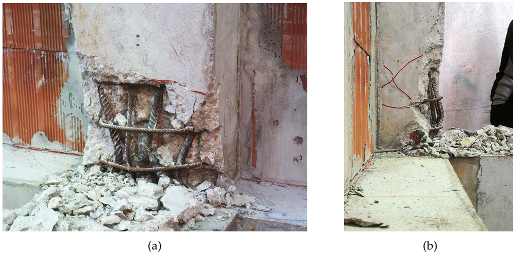
FIGURE 4.41: Final damage on beam front (a) and lateral (b) sides of J_{01\_S} – Geolite – C specimen.
