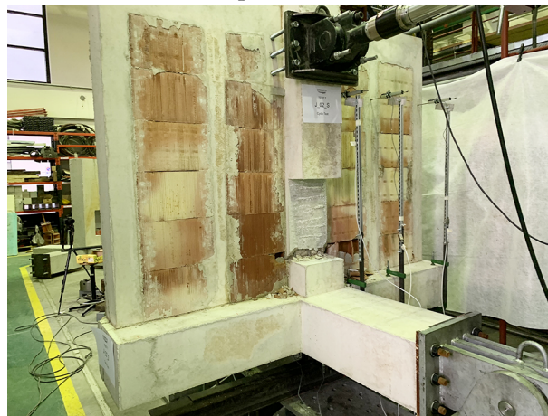
FIGURE 4.91: Final damage in the beam of J_{02\_S} - C specimen.
