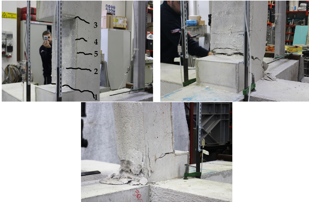
FIGURE 4.70: Crack pattern evolution in J_{02} - M^+ specimen.
