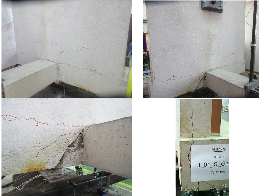
FIGURE 4.39: Crack pattern evolution on the slab side of J_{01\_S} – Geolite – C specimen.
