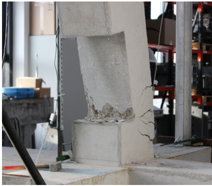
FIGURE 6.23: Crushing damage at the final stage of the experimental and numerical analysis of J_{02} - M^- specimen.
