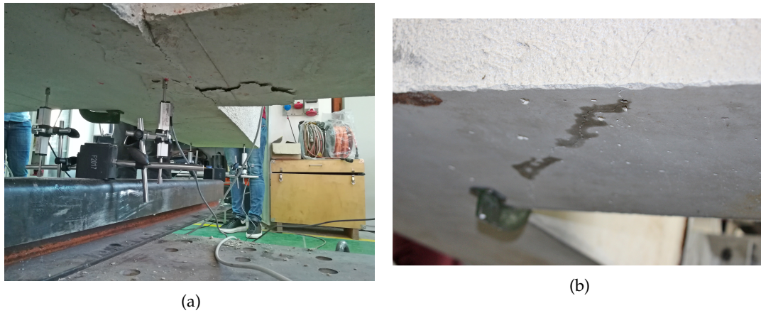
FIGURE 5.18: Joint crack pattern in J_{01\_S} - M^+ (a) and J_{02\_S} - M^+ (b) specimens.
