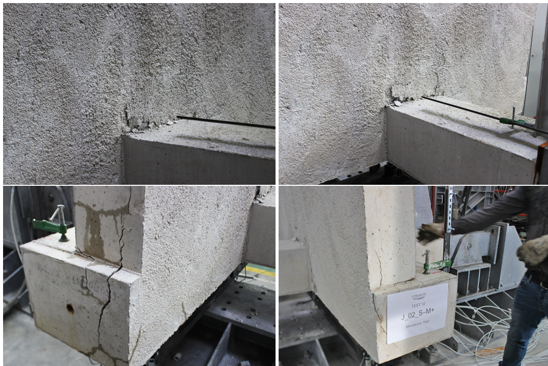
FIGURE 4.93: Crack pattern evolution on the slab side of J_{02\_S} - M^+ specimen.
