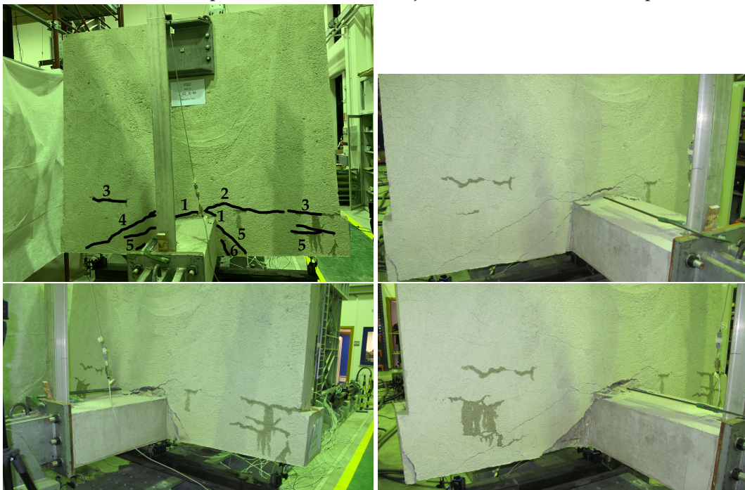
FIGURE 4.97: Crack pattern evolution on the slab side of J_{02\_S} - M^- specimen.
