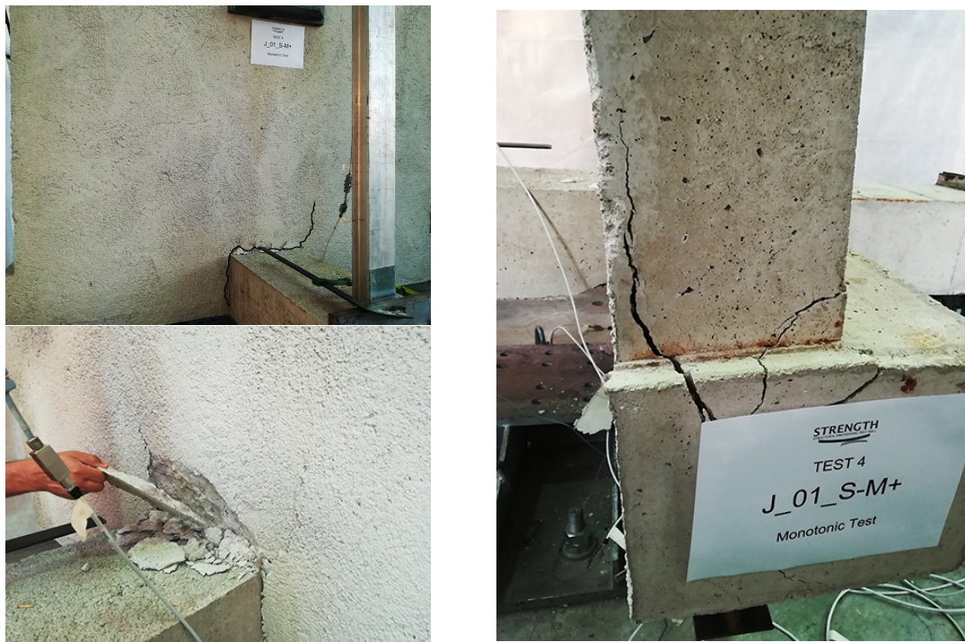
FIGURE 4.47: Crack pattern evolution on the slab side of J_{01\_S} - M^+ specimen.
