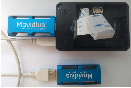
Fig. 1. One of the Movidius smart-cameras.
